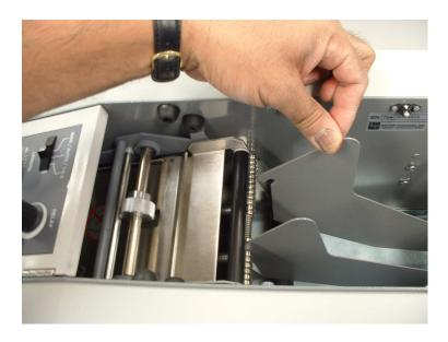
The tape roll guides in the tape basket should be properly set for the widths of tape being dispensed. The roll of tape should preferably be centered between the frames by confining the tape loosely between the roll guides which engage in between the spring loaded spacers on the tie rods.
